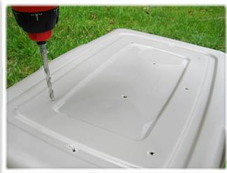
Drill/screw 8-10 small holes on bottom & lid of container
