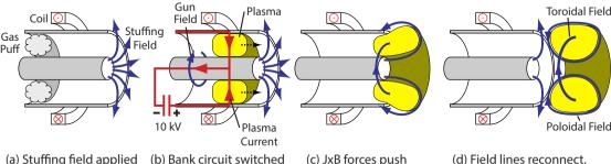
(b) Bank circuit switched (a) Stuffing field applied (c) JxB forces push by external coil, gas is on, gas is ionized plasma to the right, spheromak structure is puffed in stuffing field bulges formed
