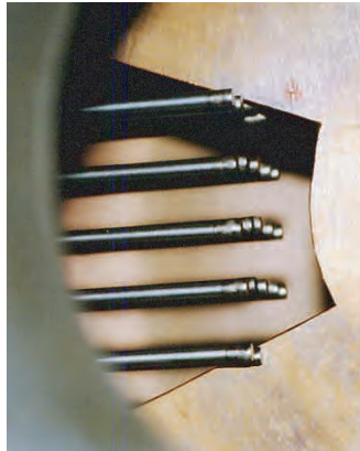
Figure 3.5: The flux conservers. A. The vacuum chamber split down the midplane reveals the conserver inside. The conserver’s two “chevron” holes can be seen. B. Looking into the port in which the 3D magnetic probe is attached. The holes visible in the conservers allow four of the five vertical planes of probe stalks (discussed in Section 3.2.1) to reach inside the spheromaks. The central plane of probes lies between the conservers. C. The 3D probe, now installed, is viewed from inside one of the conservers.
