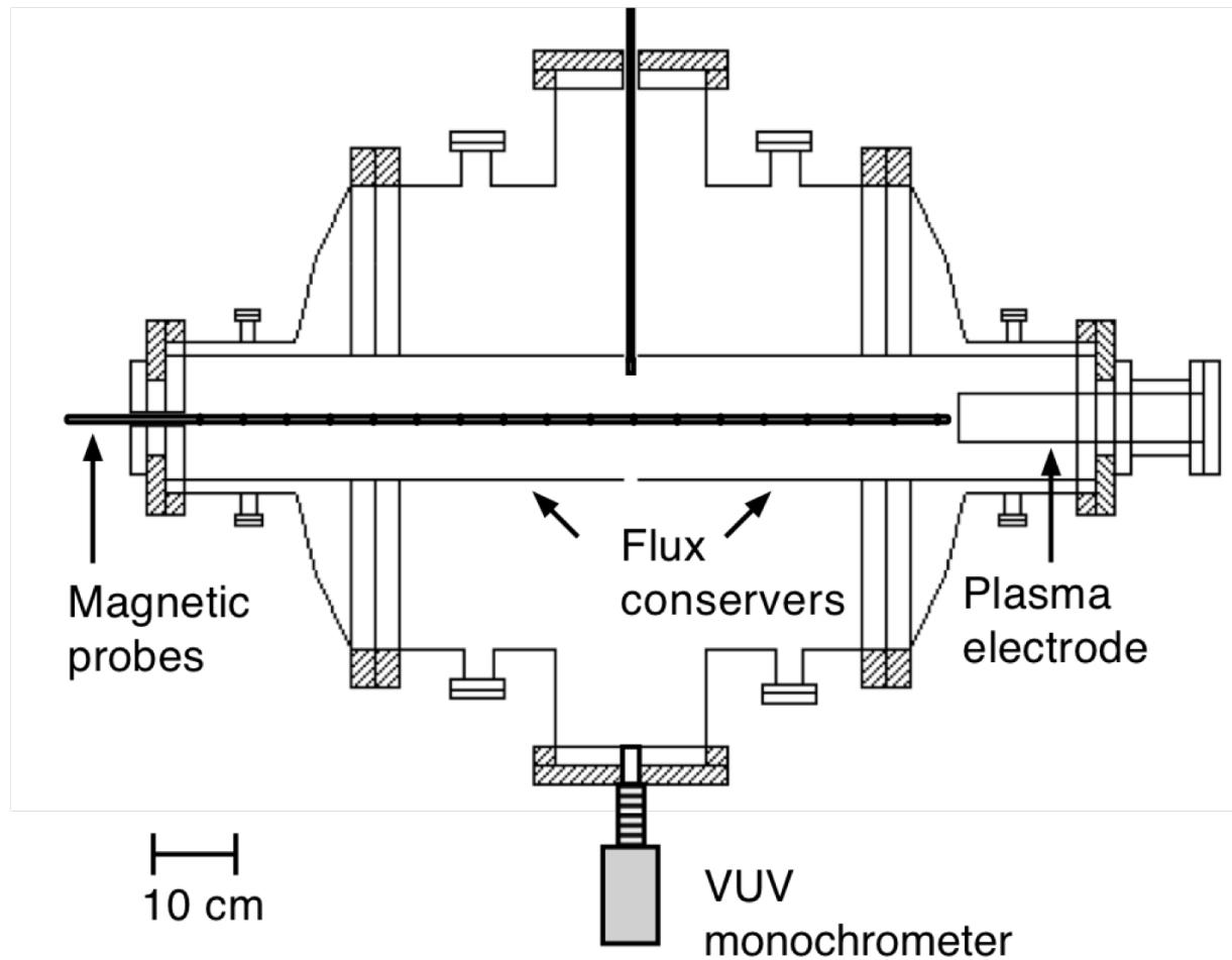
Chamber is baked and glow discharge cleaned,  $P = 10^{-8}$  torr
