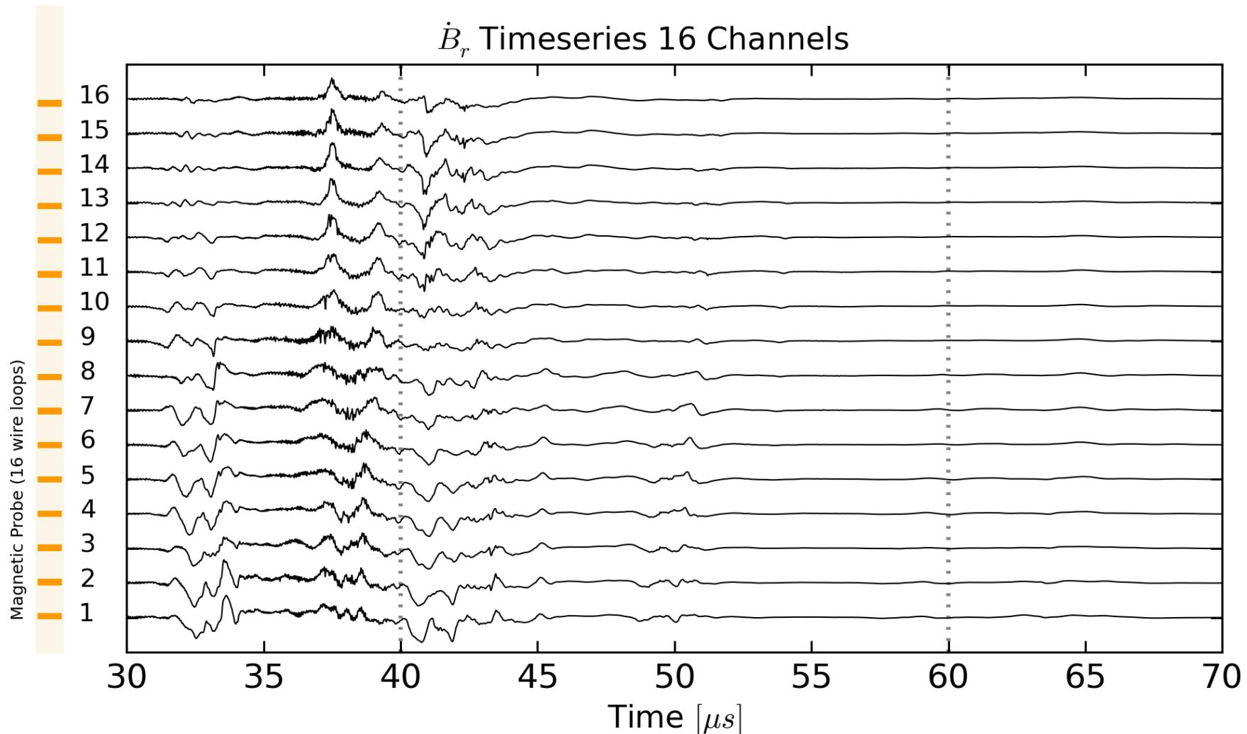
16 channels, 4 mm spacing, 65 MHz, 14 bit
