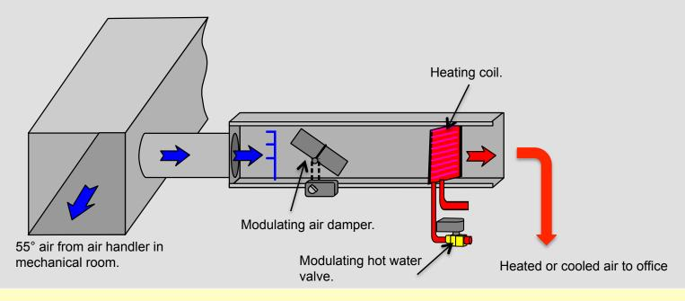
The damper opens to supply more cool air the warmer the space gets. When the space reaches temperature the damper modulates to maintain a low flow of ventilation air. When the room needs heat the heating valve opens to warm the flow of ventilation air.
