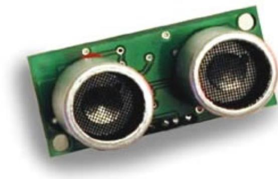
This particular sonar has a 0.866 cm wavelength, a 0.03-3 meter range of detection, and a sticker price of \$37-\$42US. The sonar requires a 5V pulse input and returns another 5V pulse output, with the length of the pulse dependent on the amount of time elapsed before a sound wave returns to the receiver. A 166Hz 50/50 pulse train was therefore applied continuously to the device. The
