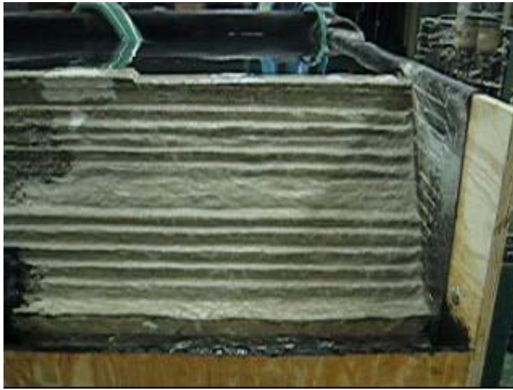
Figure 33: Nappe Flow on Dam
