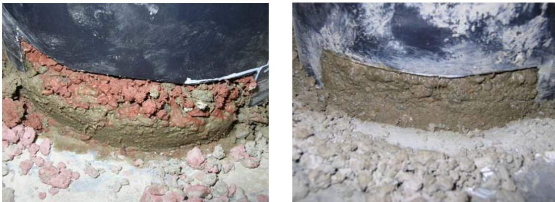
Figure 8: Lateral Deformation in Consistency Tests
