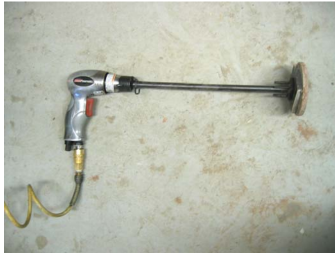
Figure 5: Pneumatic Hammer with Circular Tamping Head
