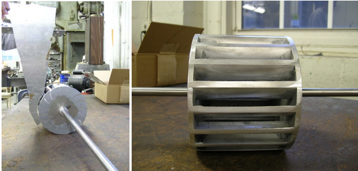
Figure 29: Completed Nozzle and Turbine.
