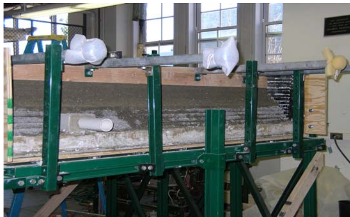
Figure 9a: Adjustable Downstream Form
