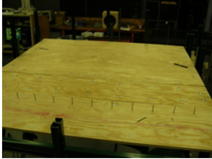
Figure 26: Top view of plywood floor of reservoir. The lines of bolts crossing the frame define the three sections of plywood.
