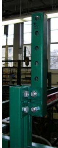
Figure 21: Column-leg and extension for sidewall support.
