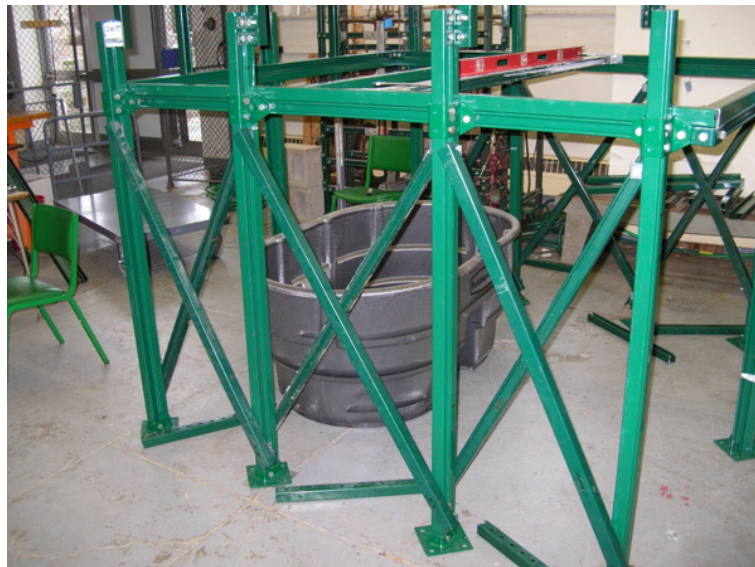
Figure 24: Cross-bracing on 7 ft side of structure.
