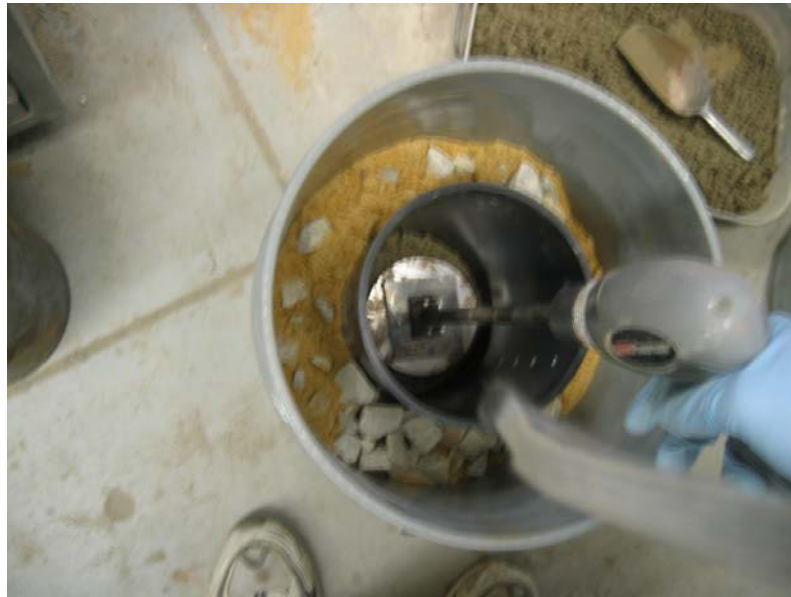
Figure 6: Compaction of Wet Density Specimens
