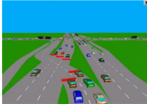
Figure 1 - Those wishing to make a left hand turn are directed into a bay between the two main lines of traffic, as seen in the middle of the figure.
