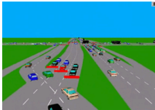
Figure 2 - The drivers then cross the oncoming lanes of traffic into a bay that is located to the left of the oncoming traffic lanes.
