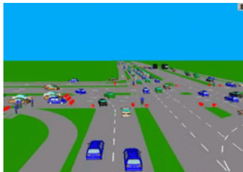
Figure 3 - The drivers then proceed to the intersection, where they make their left hand turn without having to wait for oncoming traffic to pass. The lights are timed so that soon after the green light is given to cross oncoming traffic, the light at the intersection turns green, allowing only one waiting period for left-hand turning traffic.
