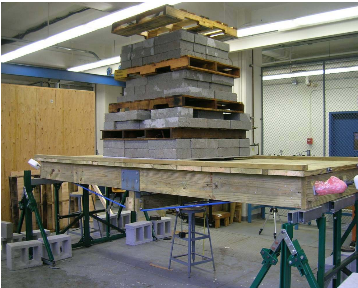
Figure 6.6: Trimetric view of Bridge Supporting Full Load
