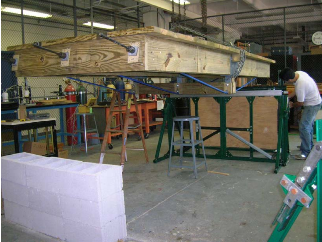
Figure 6.2: Bridge Suspended About Mid-Span Connectors During Weighing
