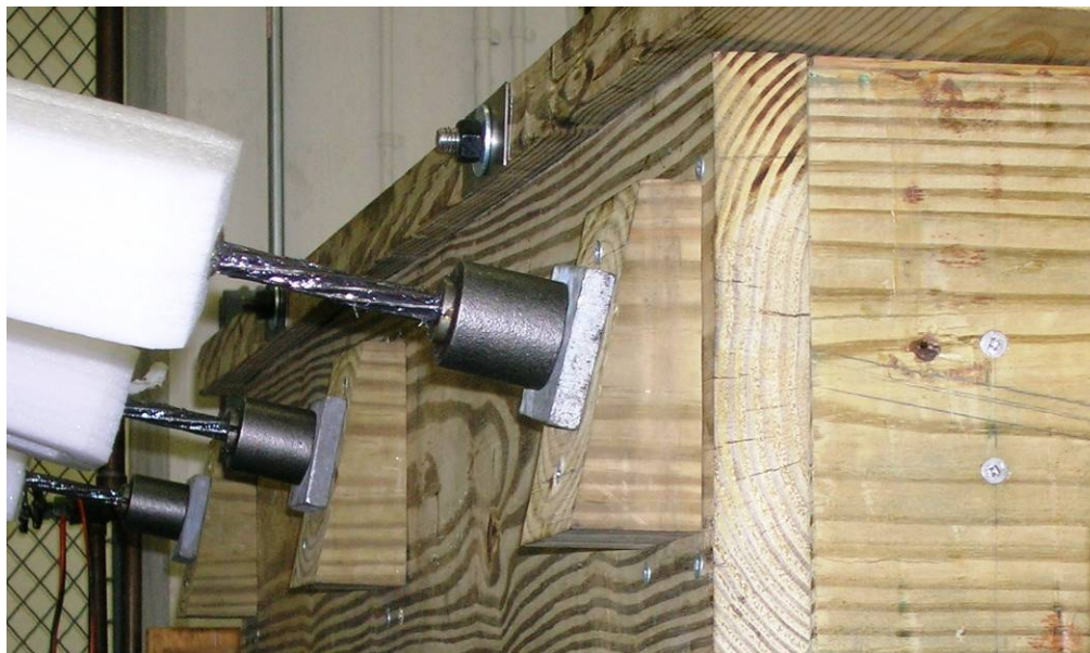
Figure 5.9: Close-up of Header Plate, Anchor Block, Cable and Anchorage
