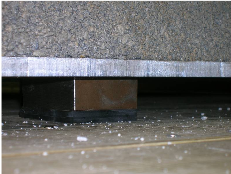
Figure 6.4: Close-up Detail of Loading Point Transfer Mechanism
