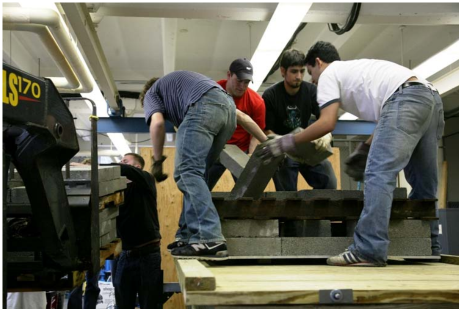
Figure 6.5: Manpowered Loading Process
