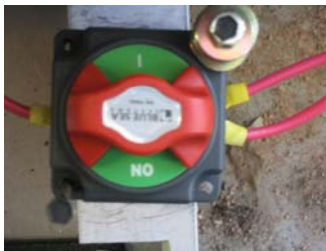
Figure 11. Knob switch selected for our go-kart.
