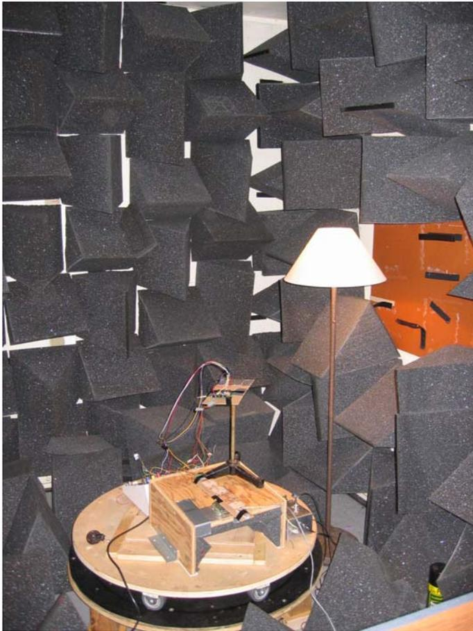
Figure 11 (left): Test setup in anechoic chamber
