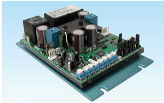
Figure 10: KBBC-24M controller for the steering actuator.
