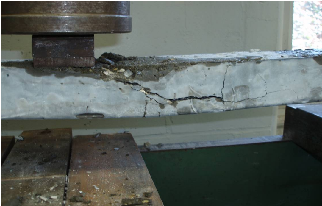
Figure 4. Shear Failure (Beam 2)
