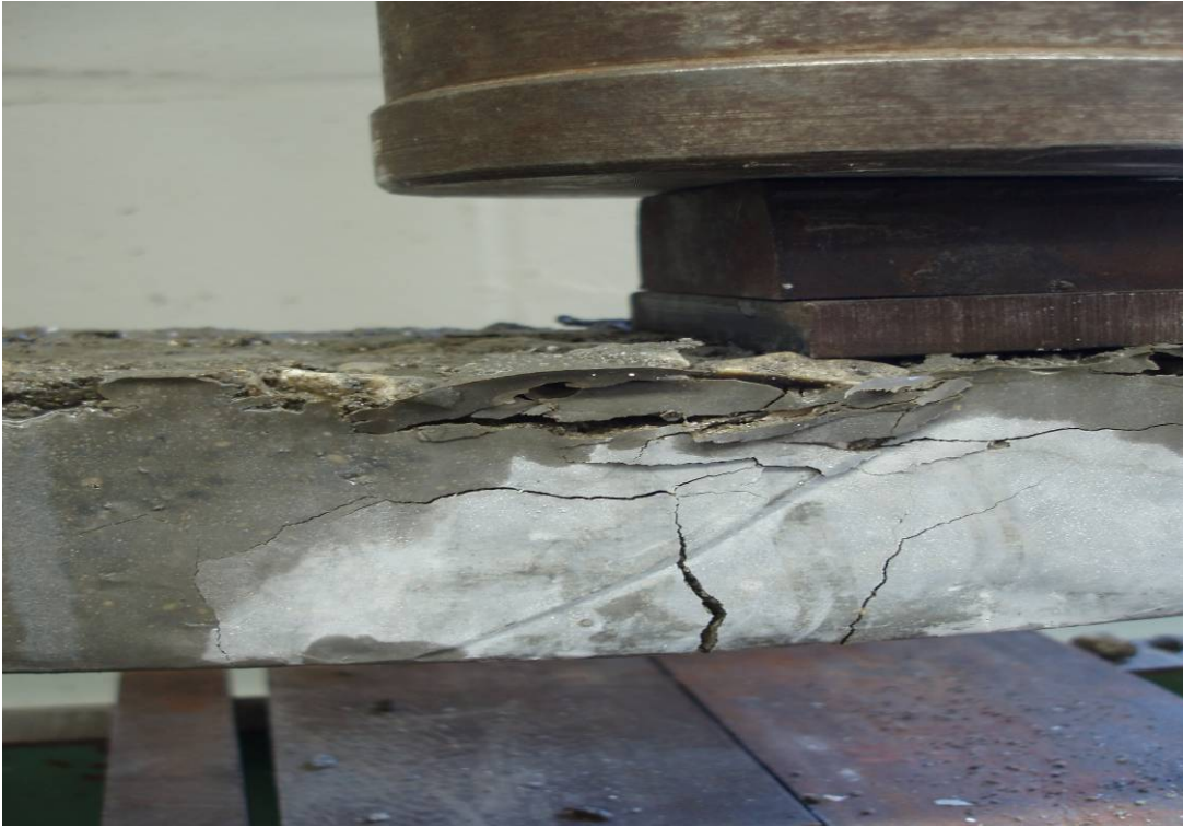
Figure 3. Crushing Failure (Beam 6)
