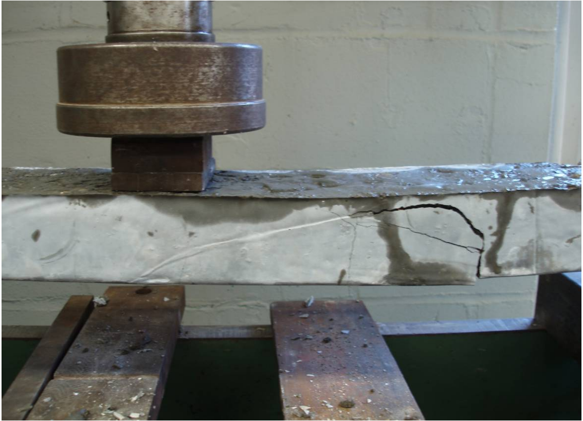
Figure 5. Bond Failure (Beam 8)
