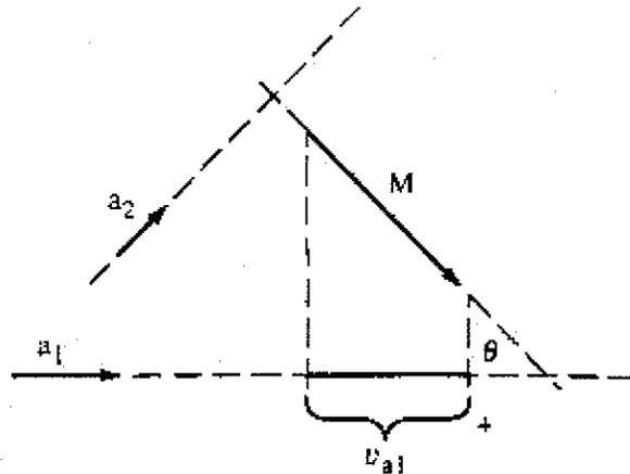
Figure 1. Lead vectors  $a_1$  and  $a_2$  in relation to the cardiac vector  $M$ .
