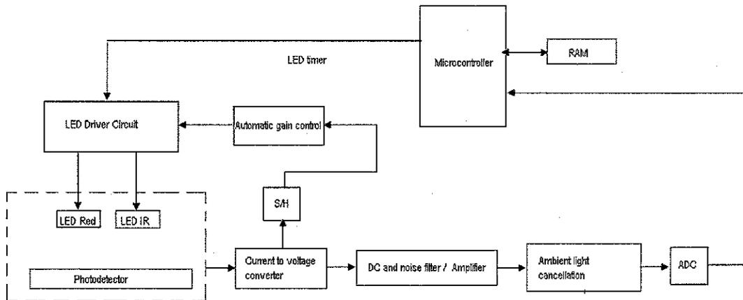
Figure 6. Block diagram for a pulse oximeter.
