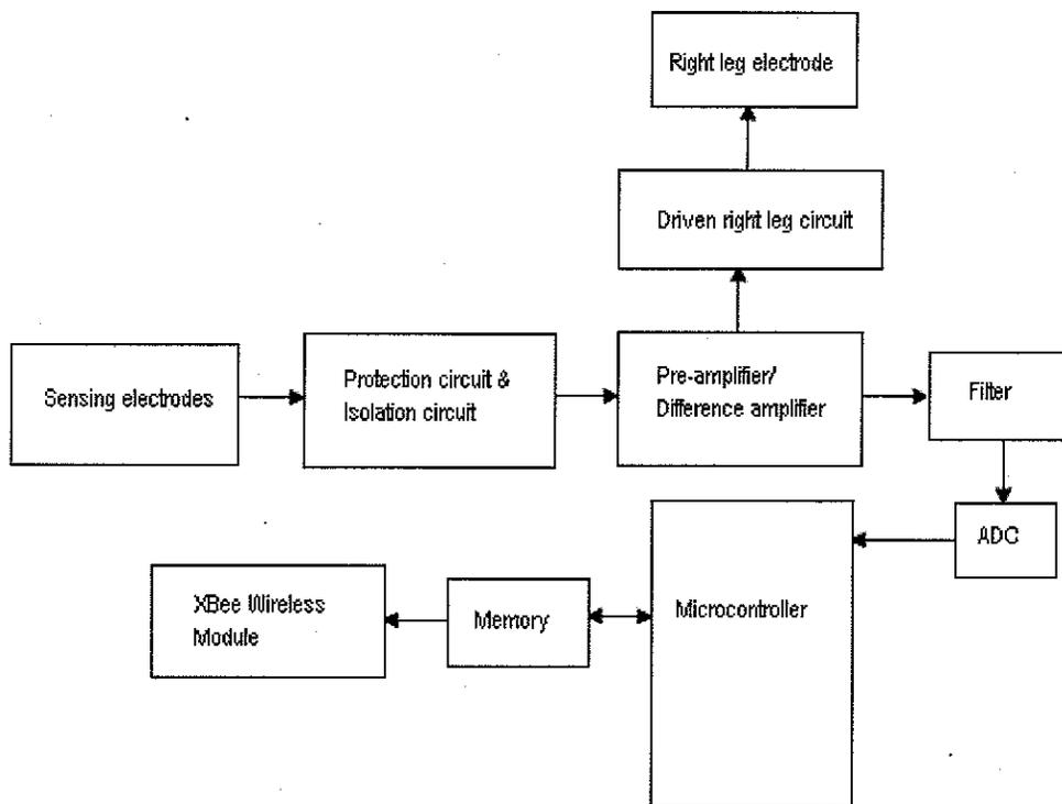
*Figure 3. ECG circuit block diagram*
