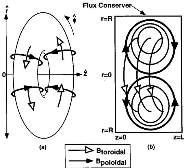
FIG. 1. Two views of a spheromak with the magnetic fields and coordinate axes indicated. The cross section at right is taken in the poloidal ( $r-z$  plane). The flux conserver is shown in the cross section view only.
