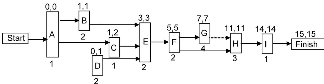
Now we're ready to find the Critical Path for this network. Any arrow connecting nodes that each have equal ES and LS values is part of the Critical Path. Nodes having unequal ES and LS values have "Slack" or "Float" time associated with that activity equal to the difference between ES and LS. There is no slack anywhere on a Critical Path - any delay or "slip" in an activity on the Critical Path results in equal slip at the Finish. Thick arrows below denote the Critical Path:
