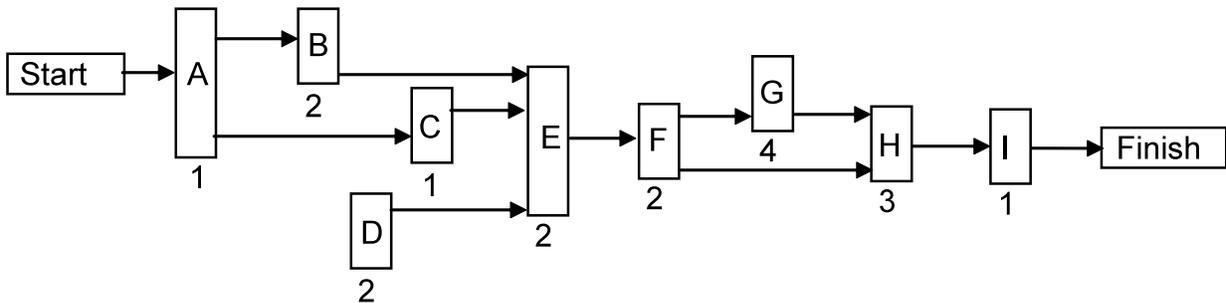
We now determine the Earliest Start Time (ES) for each activity by making a "forward pass" through the diagram from Start to Finish, beginning with ES=0 for the first activity in any branch and adding the Duration of each activity to determine ES for each subsequent activity. When multiple branches converge at a node, the latest of the possible ESs prevails.
