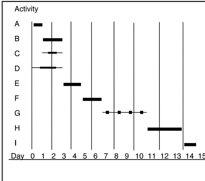
Thin lines here indicate optional activity placement (e.g. C requires 1 day between Days 1 and 3). Thick lines indicate activities that are on the Critical Path.
