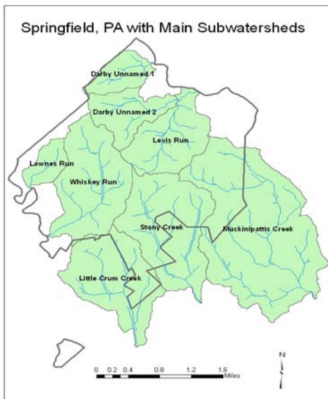
Figure 2. The eight main second-order stream subwatersheds draining Springfield that were delineated using BASINS (USEPA) and USGS digital elevation data, followed by nonpoint pollutant modeling by AVGWLF (Penn State) and, finally, prioritization for cost effective management practices by our optimization model (Swarthmore College) in this study. The boundary line of Springfield is shown as a thick gray line. Subwatershed boundaries are shown as thin gray lines. First and second order streams are shown in blue.
