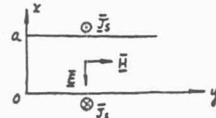
$$\underline{5.6} \quad P = \frac{1}{2} |\bar{E}|^2 \frac{Wa}{\eta} = \frac{(10^4)^2 \times 7.1 \times 10^{-3} \times 1.5 \times 10^{-3}}{2 \times 120\pi \times (1/\sqrt{2.5})} = 2.253 \text{ W}$$
