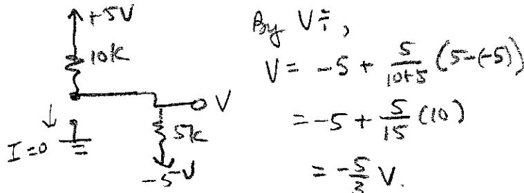
Check for  $D_2$  on as input a &  $D_1$  off ( $i_D = 0, V_D < 0$ )
