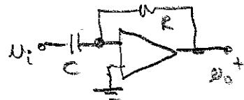
$$C \frac{dV_i}{dt} + \frac{V_o}{R} = 0 \Rightarrow V_o = -RC \frac{dV_i}{dt}$$
