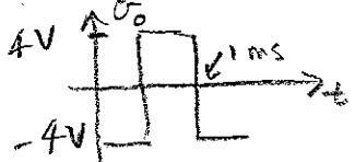
$$f = 1\text{kHz}, V_p = 4\text{V}, V_{avg} = 0$$
